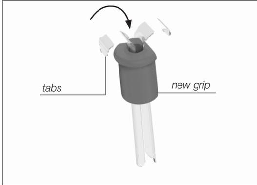
2. Place the tabs inserted into the grip at the top of the handle.
