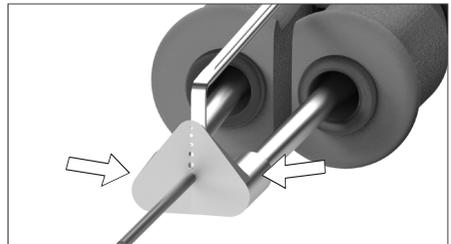
Pinch the wire with the blades according to the diameter of the wire to be stripped. The pinched area will be melted by heat.
