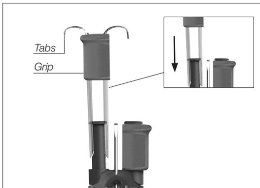
3. Push the grip with the tabs onto the handle.
