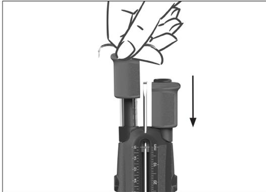
4. To remove the tabs, hold the grip and pull them out. Use pliers if necessary.
