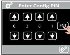
Press the configuration symbol. Enter Config PIN.
