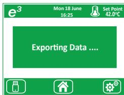
The control system will automatically upload any missing data from the last export command.
