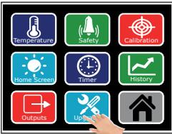
The upgrade key is password protected and used at manufacturing stage, or, to upgrade features such as Timers.
