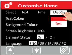
The run screen can be colour selected to suit the environment. The chamber will have default colours set depending on the model, but you can change colours to your preference. Both run screen text and background colours can be changed and as you change the colours, these are represented in the top bar. Available colours are navy blue, green, grey, black, red, light blue and white.
