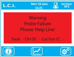
Sensor failure. If the probes are damaged, the control system shall automatically turn the heating elements off.
