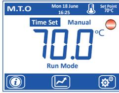
Select to run in either Real Time Clock mode or in Manual mode.
