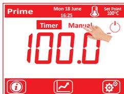
Repeat the procedure if required, or select manual mode, to go back to normal running mode.
