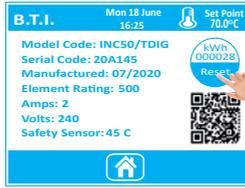
To view chamber information such as serial codes, power ratings, 2nd safety temperature value, press the **i** button, or, **e<sup>3</sup>** on E3 models.
