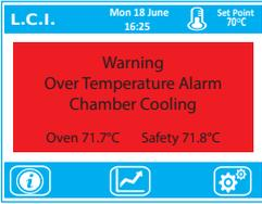
The control system is designed to indicate any faults should they occur.
