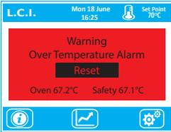
If the unit is set as Auto reset, when the temperature falls below the (Value - Hysteresis) it will automatically reset and continue operations.
