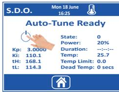
In **PID** mode, you can manually enter the P, I, and tL and tH value to optimise the control. For fan units, the P is defaulted to 3.000 and for fanless units the P value is defaulted to 1.500. The Integral and tL and tH values are best calculated using the Autotune. Please note the algorithm used in the control system uses Fuzzy Logic. This means these values are constantly updated to provide optimum control.
