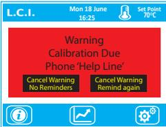
If you requested a calibration certificate with your chamber, the control system shall give you notification when the calibration is about to expire one month before. If you require a new calibration, please contact your supplier.
