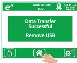
Once all transfer is done, remove the USB memory and press the
