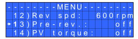
**12**) **Rev speed – Reverse speed:** You can select any reverse speed value of the screwdriver between the maximum and the minimum specific speed of every single screwdriver (see table with technical data).
