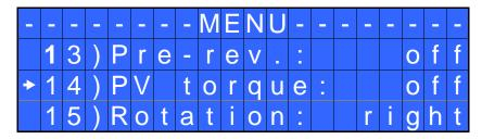
**14) PV torque:** Period of time in which the screwdriver works at maximum torque before switching to the torque that has been set by the user. You can set time from 0.1 to 10.0 sec. To disable the function select OFF by pressing  $\mathbb{Q}$  as many times as needed.
