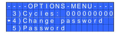
3) Cycles - Number of total screwing/errors done which have been carried out: It shows the number of fastened screws and occurred errors. This number can't be modified.
