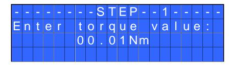
Set the torque value by selecting each digit individually pressing  $\Omega$  and  $\nabla$  and press OK to confirm it, then press OK again to save. You will see:
