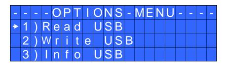
1) **Read USB**: press OK and read the USB drive and select the file SETxx.KOL you desire. The EDU control unit recognizes only files as SETxx.KOL (see EDU EXPAND part).
