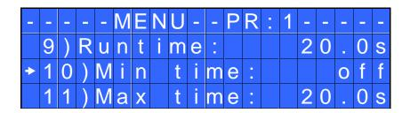
**9) Runtime**: You can set the time of a tightening, from OFF to 20.0 sec. When the pre-set time has been reached, it results in a torque signal.
