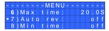
**6) Max time - Maximum time**: You can select the maximum time of tightening. You can set from 'Min time + 0.1s' to 20.0 sec.
