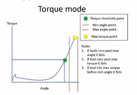
A TORQUE/INPUT (T/IN): It corresponds to *Torque* mode, except for the threshold torque which can't be set by the operator: in fact the value is the result of an external impulse through a proper contact (see paragraph "connections"). It can be very useful if the operator wants the control unit to start counting the angle from a position which is indicated by a precision instrument.
