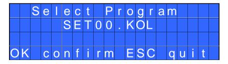
2) **Write USB:** press OK and create your new SETxx.KOL application where you save all the parameters you have set in the control unit.
