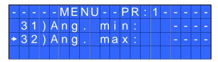
**32) Ang. max** - **Maximum angle:** Maximum angle threshold. You can set it when T&A is set on Tor, T/in or T/lv (see T&A specific instructions). The maximum angle the operator can set is 29999°.
