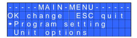
**Program setting**: It indicates the menu section where you can set or modify the fastening parameters.
