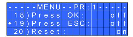
**18**) **Press OK:** when ON, press OK at the end of each screwing. When OFF, the control unit resets automatically after a screwing.
