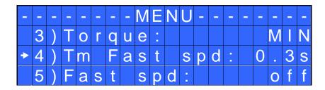
3) **Torque:** you can select the desired torque as a percentage of the torque range of the selected screwdriver. For example, for a Pluto10, a 50% setting will result in a torque in the area of 4.5 Nm. The torque range is always referred to the MAX speed. In case you're not working at maximum speed, the torque range will
