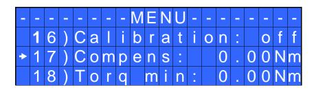
**16**) **Calibration:** ON allows to see the torque value on the main screen. OFF doesn't show the torque value.
