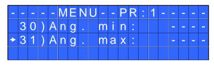
**31) Ang. max - Maximum angle:** Maximum angle threshold. You can set it when T&A is set on Tor, T/in or T/lv (see T&A specific instructions). The maximum angle the operator can set is 9720°.
