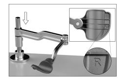
Fit the tool arm onto the base and tighten the screw.
