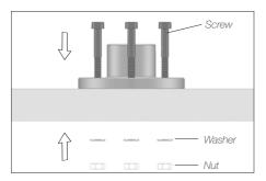
Fix the flange on your work table with the supplied screws, nuts and washers.
