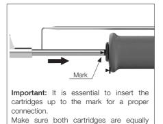
**W440 cartridges** have a proper centering to ensure a good functionality. Before tightening the screws, align the cartridges in working position using a flat pliers (Ref. PLR-195).
