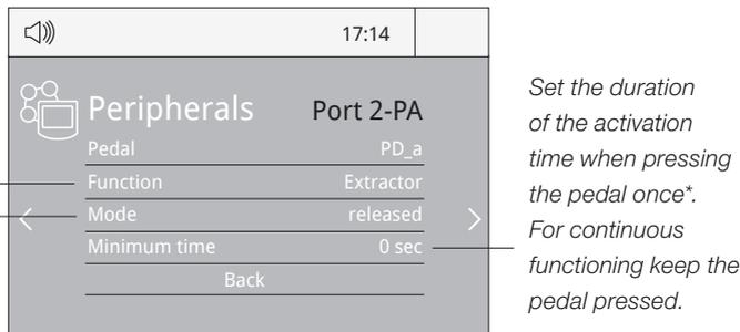
\*NB: The same can be applied inversely when continually pressing the pedal and releasing to activate.
