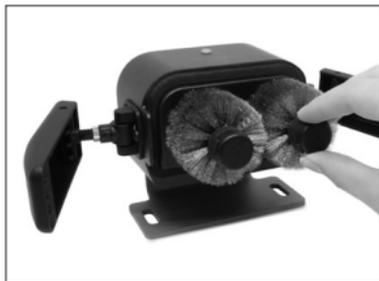
4. The Splashguard also works as tin collector. Clean it and place it back in its position.
