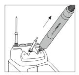
Place the cartridge in the extractor and pull the handle to remove the cartridge.
