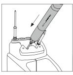
Place the handpiece on top of the new Cartridge and press down slightly.
