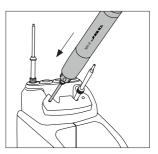
Use the holes to push and fix the cartridge in its final position.
