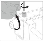
1. Remove the 4 clamp knobs and the 4 black rubber caps.
