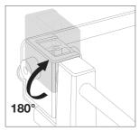
2. After removing both guides, turn 180° the guide supports.
