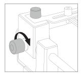
3. Place the guides, the rubber cups and adjust the sliding clamp knobs again.
